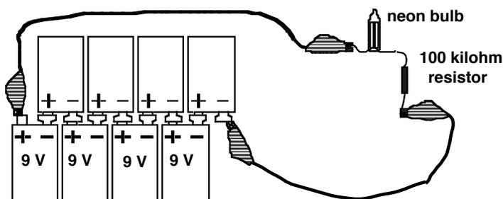
Figure III.6.1 Neon bulb and 9V batteries
