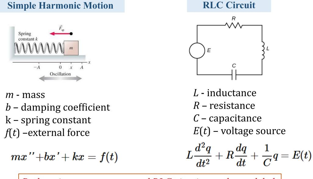
Both spring-mass systems and RLC circuits can be modeled by second-order constant-coefficient differential equations.
